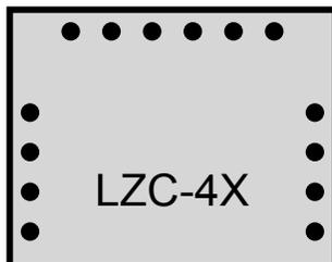
The LZC-4X photoreactor is equipped with 6 top lamps, and 8 side lamps.
