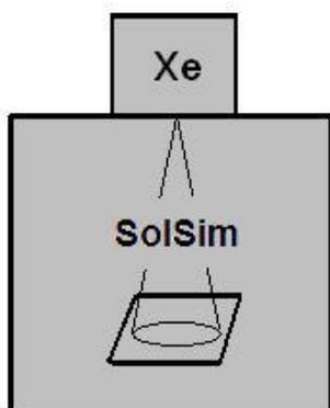
The SolSim utilizes a Xenon lamp placed at the top of the photoreactor chamber along with a custom filter assembly. The solar simulation filters are placed on a stand 3" above the chamber floor, with samples beneath.
