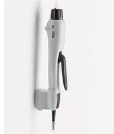
The functional, ergonomically-designed hand controller is fully autoclavable. Pressing the lever allows fine adjustment of the suction power and permanent suction can also be enabled. The continuous tubing prevents contamination of the interior of the hand controller. Adapters for pipettes and pipette tips (200, 300 and 1000  $\mu$ l) and a wall mount are supplied with the hand controller.
