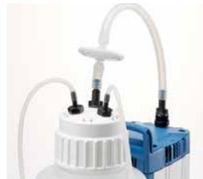
Autoclavable, self-sealing quick couplings allow safe decontamination of biological risk material.
